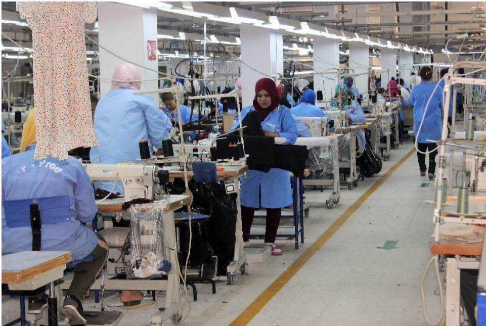
Designated work spaces were marked at TF PROD as party of Kaizen Implementation thereby improving productivity
