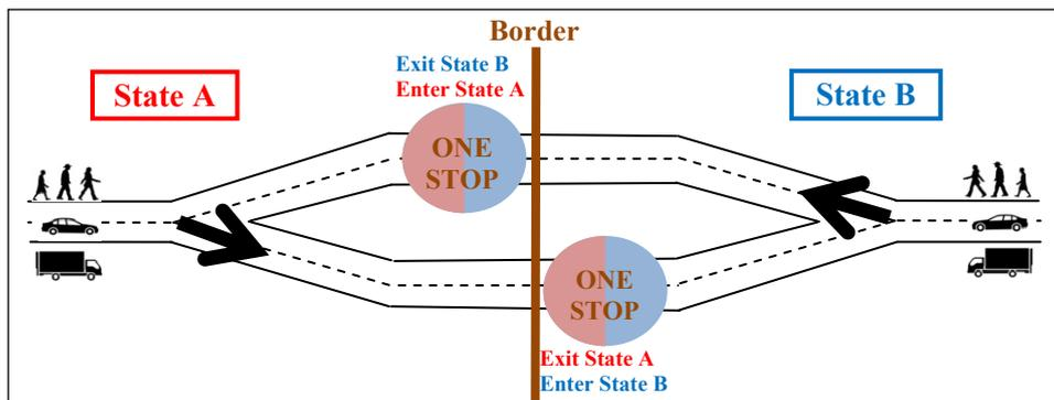
**Figure 5: Schematic Diagram of a Straddling OSBP**
